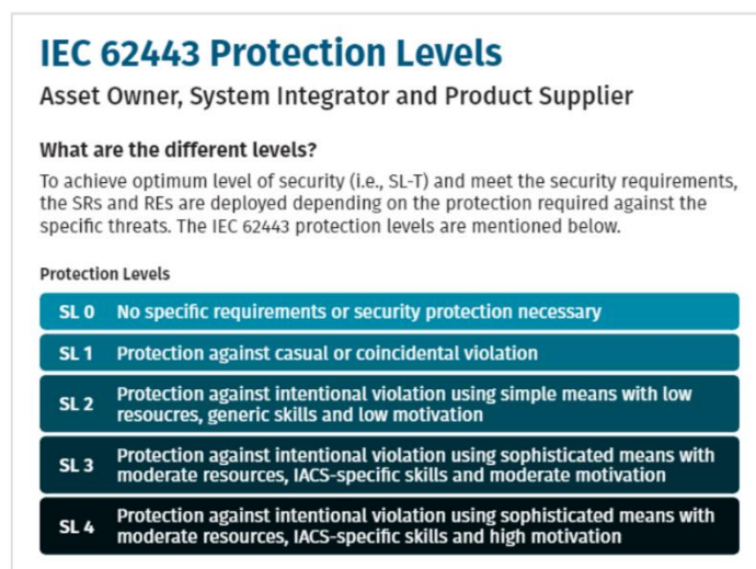
Figura 112: IEC 62443 Protection Levels
